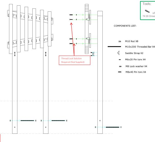
Thread Lock Solution Required (Not Supplied)
