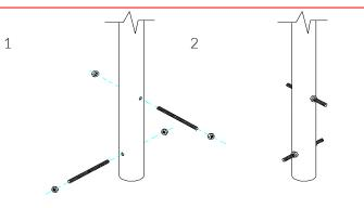
Insert M10x 150 Threaded bar into pre drilled holes in Ground Fixing Post
